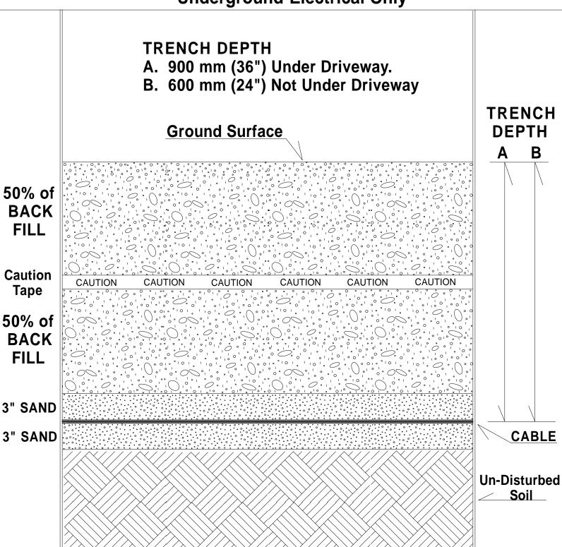
Lay cable with 75 mm (3") of sand below and above cable, back fill trench aprox 50%, then lay yellow or red caution/danger tape, then complete back fill to surface.
