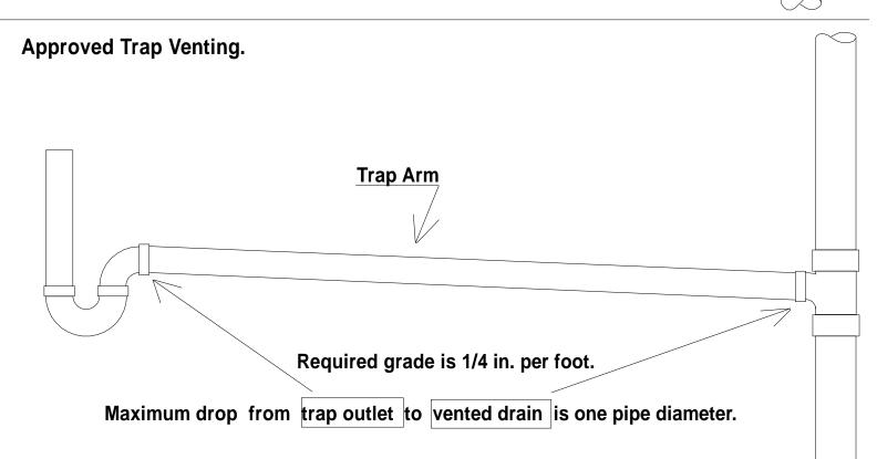
The maximum distance from trap outlet to vent, or vented drain, is determined by the size of the trap arm. Example, a 1 1/2 in. diameter trap arm, grading at the required 1/4 in. per foot, the maximum distance to the vent or vented drain, would be 6 ft. (as there are 6, quarter inch segments in 1 1/2 inches).
