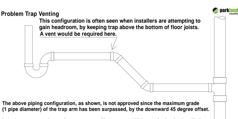
In order to meet code requirements an auxiliary vent would be required to be installed upstream of the first 45 degree elbow, offsetting down, as pointed out above.
